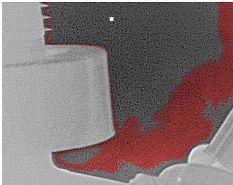
***Our proprietary HyPAT software uses false color to highlight the gas leak***
